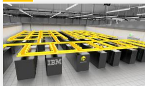
SuperMUC: IBM IDPX at GCS partner LRZ, >155 000 cores
