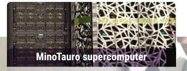
Heterogeneous cluster with NVIDIA GPUs. 343.74 teraflops top speed.
