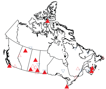
Trends of monthly mean soil temperature across Canada in May at a depth of 100 centimeters for the period 1958–2008. Red and blue triangles show positive and negative trends, respectively. Solid triangles indicate trends significant at the 5% level.
