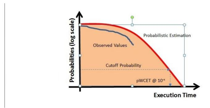
This research line covers a novel way to fulfil the timing requirements of current and future multicore-based real-time systems based on (1) injecting randomisation into the timing behaviour of hardware and software; and (2) developing probabilistic timing analysis techniques.
