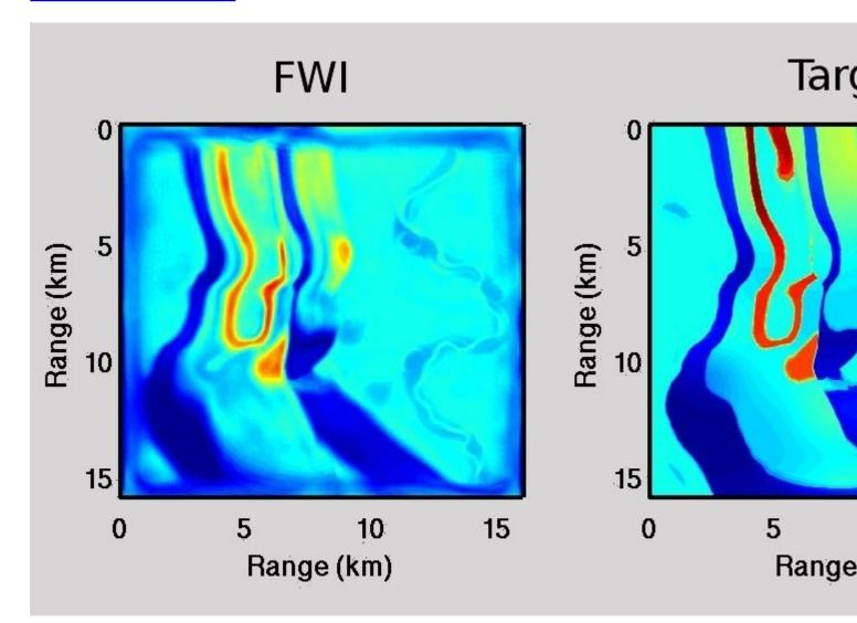
Inverse modelling gives answers to the question: What are the physical properties of the Earth? By matching recorded data with the outcome of large and complex 3D simulations we obtain accurate maps of the properties of the subsurface.
