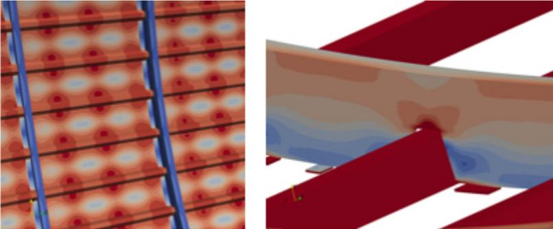
Our multi-physics parallel code Alya simulates non-linear solid mechanics for complex problems. With measured linear scalabilities in more than 100K cores, the solid mechanics module is used in several application areas: aerospace, biomedical, etc.
