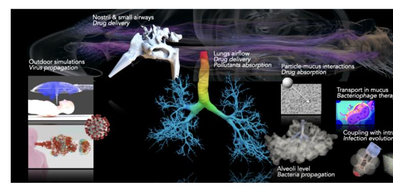
The project aims at predicting particle deposition in the respiratory system, drug delivery being the main target application. To this end, direct numerical simulation of the airflow and Lagrangian particle transport are carried out in the large and small airways.
