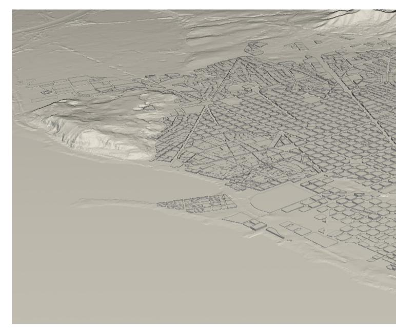
Urban-scale wind and atmospheric dispersal modeling using CFD and mass-consistent approaches. Automatic city meshing including buildings and underlying terrain. Air quality mapping based on sensor deployment and linearized CFDs at city scale.
