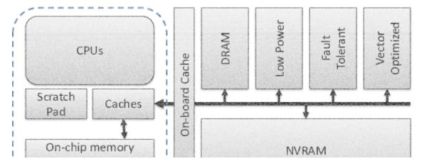
Although the exact approach to efficiently exploit heterogeneous memory systems is still uncertain, a software ecosystem clearly is required in order to assist in an efficient data distribution. We address this problem at the memory object granularity.
