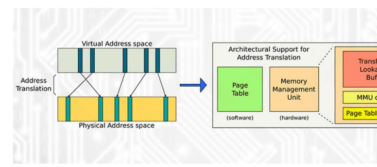
Virtual memory provides many important benefits by introducing an indirection level between the virtual address space that the process sees and the physical memory that the operating system manages. However, virtual memory introduces high overheads that we seek to reduce in this project.
