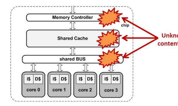
We develop new methods to derive reliable Worst-Case Execution Time (WCET) bounds for programs running in Commercial-off-the-shelf (COTS) multicore processors with unknown interference in the access to hardware shared resources.
