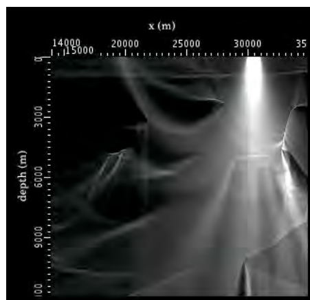
Figure 6: Imaging condition by cross-correlating source and receiver wave-field for 20 shots from the synthetic 2004 BP data.
