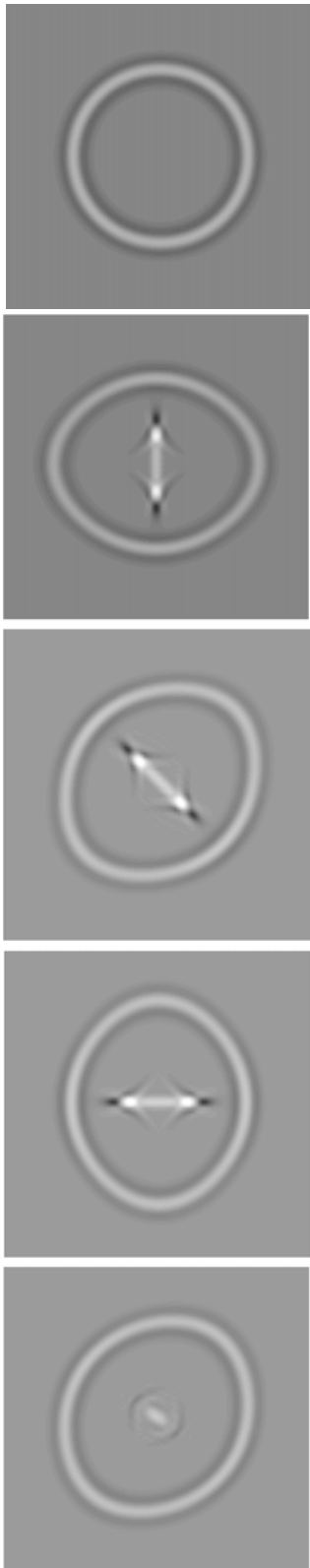
Fig 1. Impulse response for modeling. From top to bottom, they correspond to isotropic media, 3D TTI media with angle combinations \theta=\varphi=0 (VTI), \theta=45;\varphi=0 , \theta=90;\varphi=0 , \theta=\varphi=45 degrees
